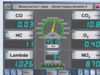
Measurement value overview. Functional display of all measurement values (here with RPM and oil temperature function/ NOx measurement optionally available).
