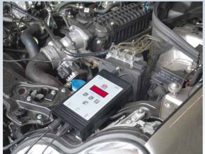
RPM VC 2, RPM measurement via vibration sensor or on-board voltage ripple effect.
