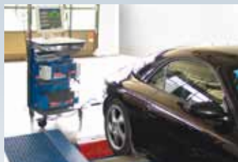
Connection to LPS function and performance dynamometer.
