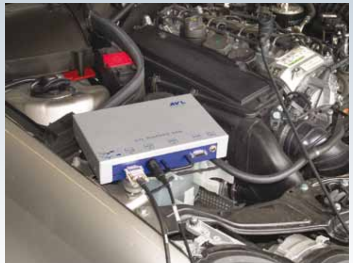
DISPEED 490, practice-oriented RPM measurement via magnet combi-sensor.
