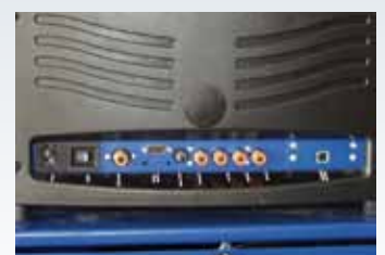
MGT 5 ASM backside: 2-point calibration (High-, Low-, and zero gas).
