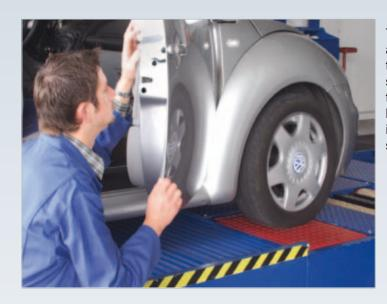
The controller enables individual switching of test plates as well as simultaneous activation of both plates. In addition, the frequency can be changed independently at each side by the operator. Due to extremely quiet operation of the tester, noises that arise during the simulation process can be detected and localised without problem. After the fault is rectifi ed, the success of the work can be checked by the same simulation.
