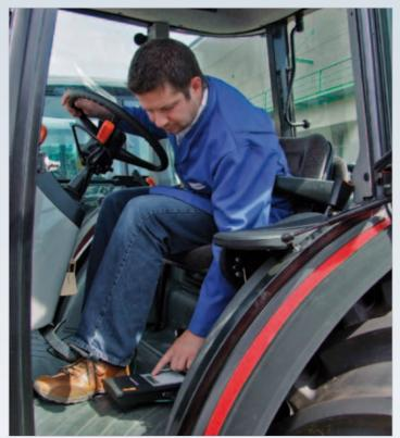
The VZM 300 measurement unit is simply placed on the  ${\it fl}$  oor of the vehicle for the measurement
