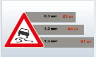
The tread depth measurement makes a significant contribution to the increase in traffic safety. As the tread depth decreases, the risk of aquaplaning increases. A regular check is essential for safety reasons.
