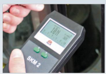
The measured values are output via a lit LCD display. The effective force and the peak force reached is represented. When switched on, the SKM 2 checks the measurement electronics independently and performs an automatic zero balance.
