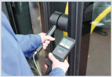
The activation forces at power-activated equipment can be checked with the closing force sensor. The application area includes doors at the bus and track, lifts, cableways, electrical activated window as well as sliding roofs, etc.
