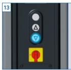
Upper end position or photoelectric ceiling barrier reached. Only lowering is possible. Lower button lights up blue.
