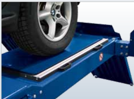
Precision slide plate (optional, available only for version "W"); Very small breakaway torque of 5 Nm and very small slide force of 15 N required at 500 kg wheel load, large amount of steel balls, hardened running surface, collector channels for dirty water.
