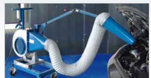
Additional blower for components
