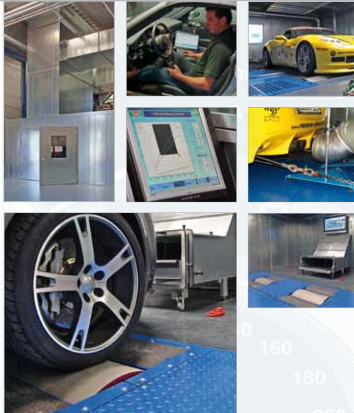
Custom equipment with soundproofing cabin, ventilation system including cooling blower and suction facility for the company Abt Sportsline GmbH
