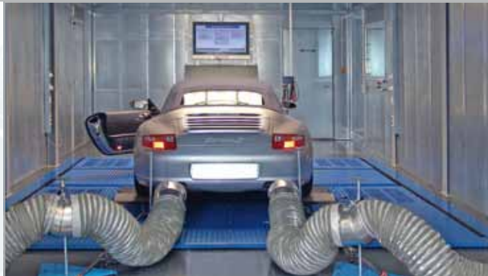
Custom equipment with soundproofing cabin, ventilation system including cooling blower and suction facility for the company Abt Sportsline GmbH
