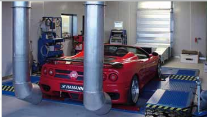
Custom equipment with soundproofing cabin, ventilation system including cooling blower and suction facility for the company Hamann GmbH
