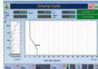
Driving cycles Reconstruction of different cycles as possible (NEFZ, ECE ...) (driving cycle expansion pack option).
