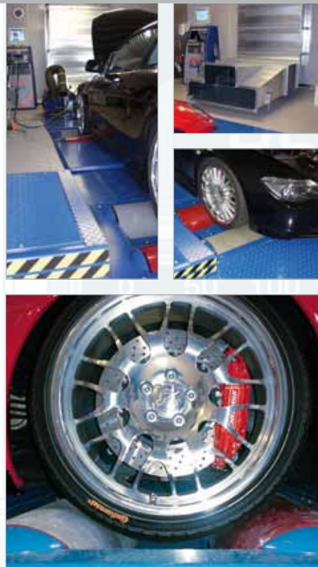
Custom equipment with soundproofing cabin, ventilation system including cooling blower and suction facility for the company Hamann GmbH
