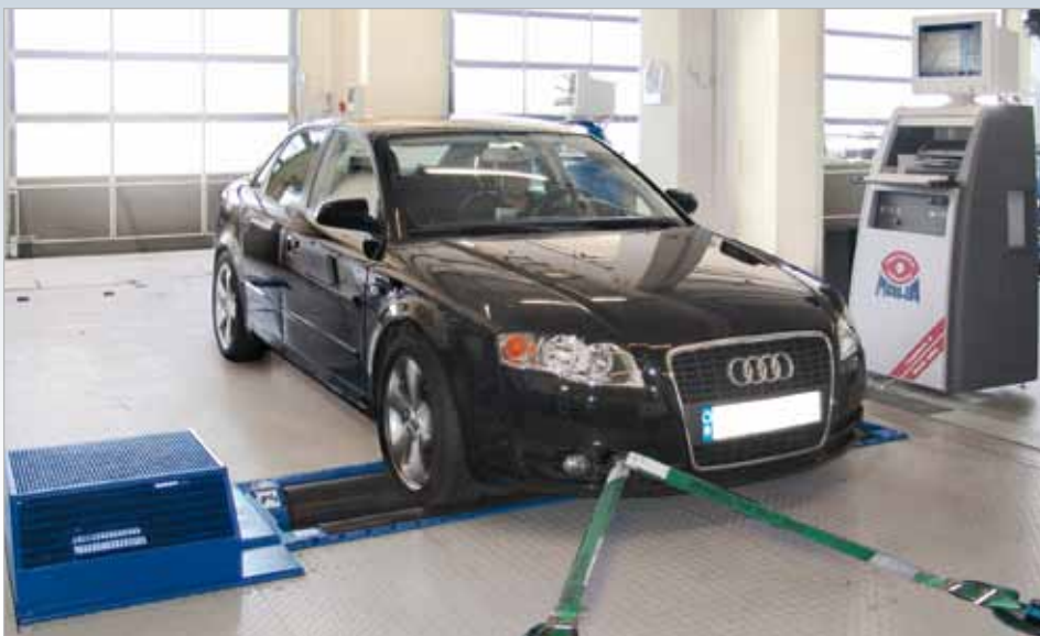
Holding the vehicle in place through tension belts.
