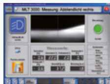
Light test Digital determination of the headlight setting by means of a CMOS camera.
