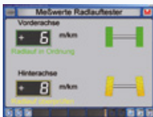
Side slip test Clear display of the directional stability of the vehicle axles.
