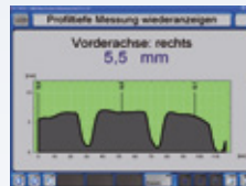
Tire tread measuring device TM 1000: Automatic measurement of the full tire tread (circumference and tire width).
