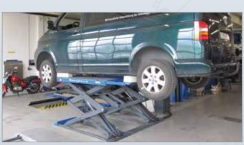
Very long extension length of the lifting plates (1550 – 2100 mm), making lifting of smaller vans possible.
