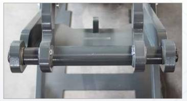
High lateral stability due to heavily dimensioned scissor arms
