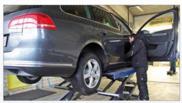
The vehicle doors of the lifted vehicle can be completely opened. The free side access to the vehicle offers comfortable working conditions.
