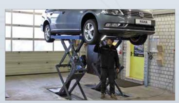
The generous lifting height allows comfortable working even with surface mounting of the TWIN F IV  $3.0/3.5~\rm U.$
