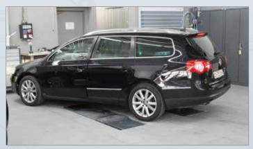
The flush-floor installed TWIN F can be driven over crosswise for maneuvering in tight entry areas.
