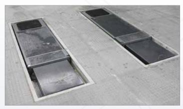
Due to foundation compensation boxes (which come standard with the TWIN F IV 3.0/3.5 U), both extensions of the flush-floor installed twin scissors lift can be length adjusted even when the lift is fully retracted. In this way the lift can be completely lowered without having to push in the extensions.
