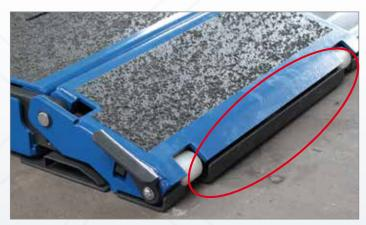
Secure locking of the extension flaps to drive over the lift (TWIN F IV 3.0/3.5~A)
