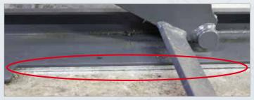
Hot-dip galvanized shim plate (comes standard with TWIN F IV  $3.0/3.5~\rm U$ ) protects the floor frame from direct contact with dirty water, adding corrosion protection.
