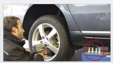
The lifting plates can be used as a practical tray for parts.
