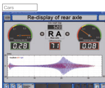
Shock absorber Test Clear graphical and digital display of measurement values
