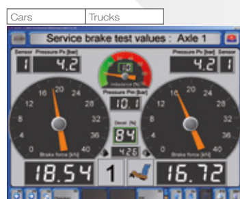
Brake test During the brake test, all relevant data are presented clearly. In addition, the various braking force parameters are displayed digitally.
