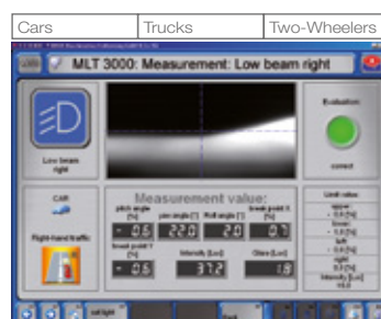
Headlight Test Digital determination of headlight setting by means of CMOS camera
