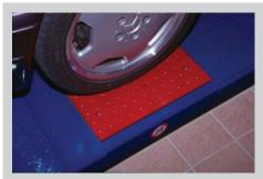
PMS model 3/X can be integrated into the sides of an inspection pit or the runways of a DUO scissors lift. The other models are recommended for usage in combination with an inspection pit.
