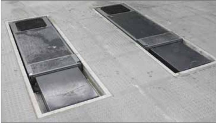
Due to foundation compensation boxes (which come standard with the TWIN F IV 3.0/3.5 U), both extensions of the flush-floor installed twin scissors lift can be length adjusted even when the lift is fully retracted. In this way the lift can be completely lowered without having to push in the extensions.
