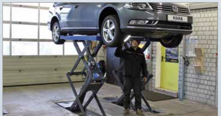
The generous lifting height allows comfortable working even with surface mounting of the TWIN F IV 3.0/3.5 U.
