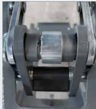
Innovative cylinder raising support: the complete lifting force is already available at the lowest lifting range. The lift retracts gently and noise-free into the lowest position, and lifts slowly and gently out of the lowest range avoiding impact on the vehicle. The cylinder raising support conducts a pure rolling movement and is maintenance- and wear-free.
