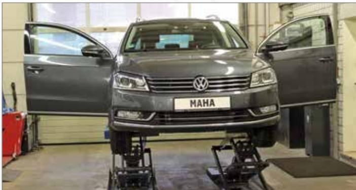
The vehicle doors of the lifted vehicle can be completely opened. The free side access to the vehicle offers comfortable working conditions.
