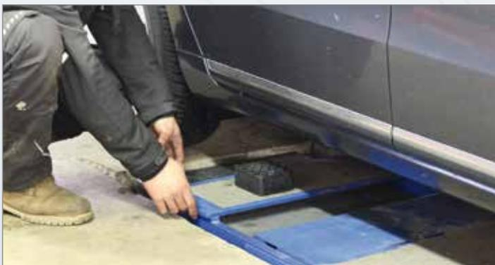
Continuously extendable lifting plates offer high user comfort - no vehicle pushing for adjustment needed.
