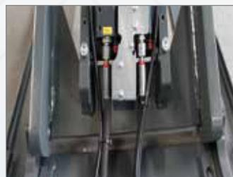
The stroke travel of both cylinder pairs on each scissor side is measured via cable pull potentiometer, the hydraulic synchronization is conducted automatically by the control. The operator is freed from manual leveling compensation. The cable pull potentiometer corresponds with protection class IP 54, the cable is protected by a pipe preventing moisture and dirt contact.
