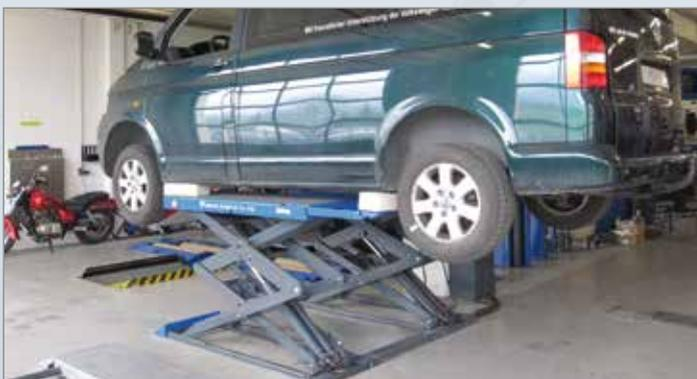
Very long extension length of the lifting plates (1550 – 2100 mm), making lifting of smaller vans possible.
