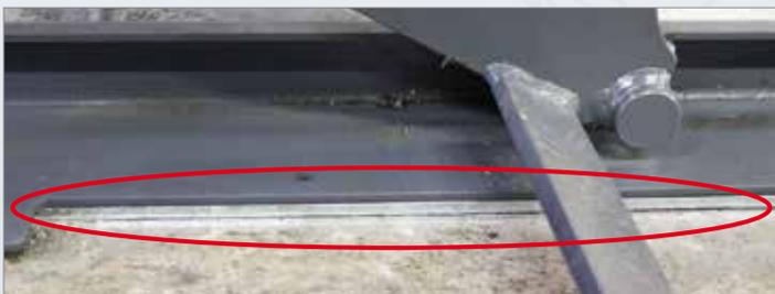
Hot-dip galvanized shim plate (comes standard with TWIN F IV 3.0/3.5 U ) protects the floor frame from direct contact with dirty water, adding corrosion protection.
