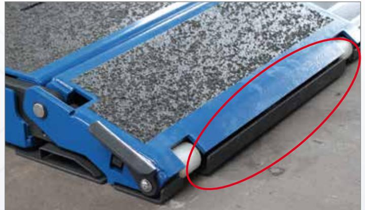
Secure locking of the extension flaps to drive over the lift (TWIN F IV 3.0/3.5 A)
