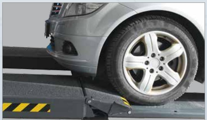
... reduce the drive-on height to 65 mm: easy access for vehicles with low ground clearance
