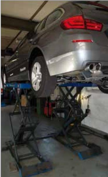
The twin scissor lifts of the TWIN F series are space-saving, making them very efficient.
