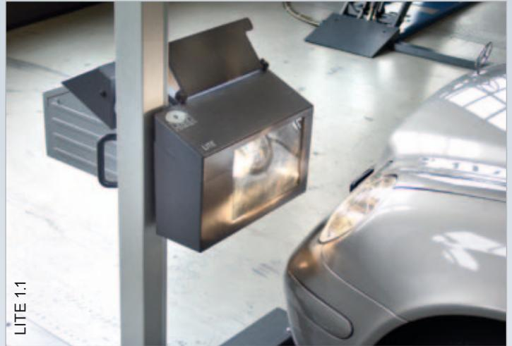
Due to the large scale Fresnel lens of the "LITE 1.1" multiple light sources can be tested without constant new positioning. Additionally, the robust version with a light weight design offers a high quality and ergonomic design.
