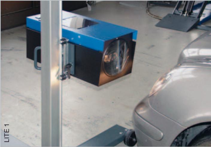
Even the low cost version "LITE 1" offers the highest precision with an aluminum guidance column in conjunction with the solid frame.
