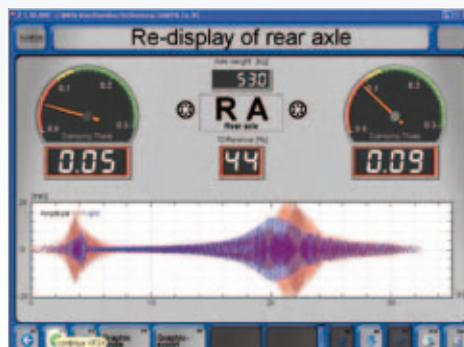
Significant representation of defective axle damping (example)
