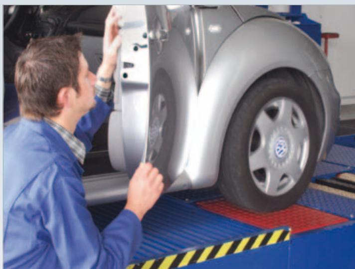
The controller enables individual switching of test plates as well as simultaneous activation of both plates. In addition, the frequency can be changed independently at each side by the operator. Due to extremely quiet operation of the tester, noises that arise during the simulation process can be detected and localised without problem. After the fault is rectified, the success of the work can be checked by the same simulation.
