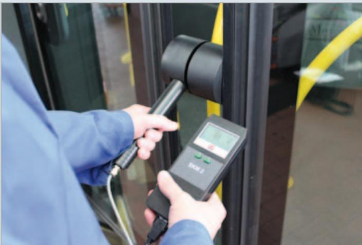
The activation forces at power-activated equipment can be checked with the closing force sensor. The application area includes doors at the bus and track, lifts, cableways, electrical activated window as well as sliding roofs, etc.
