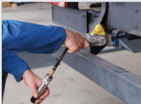
Cable and hose-free pressure transmission of measurement values via radio pressure sensor
