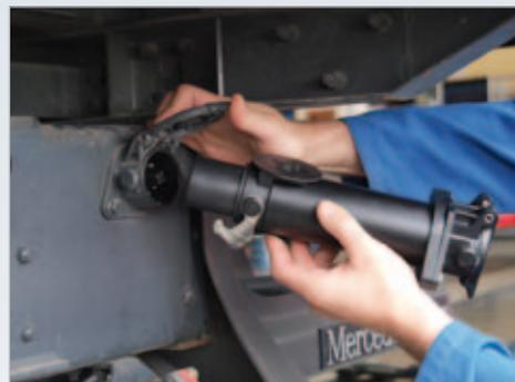
Function test of electronic trailer interface ISO 11992
