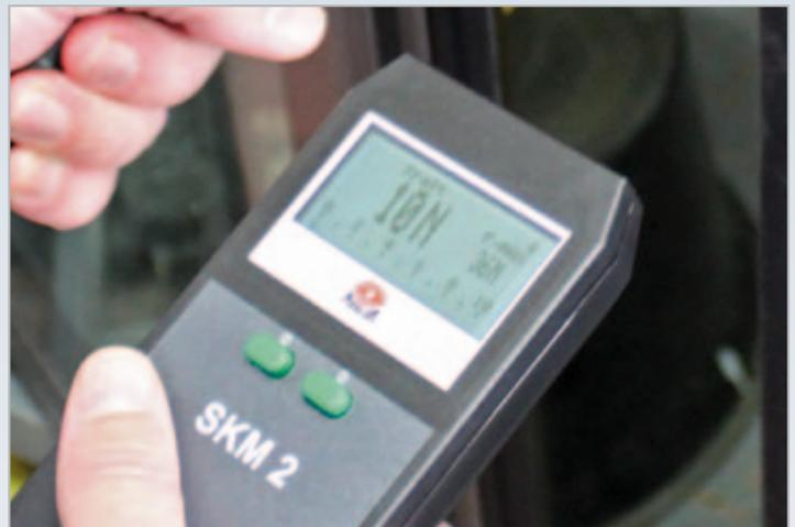
The measured values are output via a lit LCD display. The effective force and the peak force reached is represented. When switched on, the SKM 2 checks the measurement electronics independently and performs an automatic zero balance.
