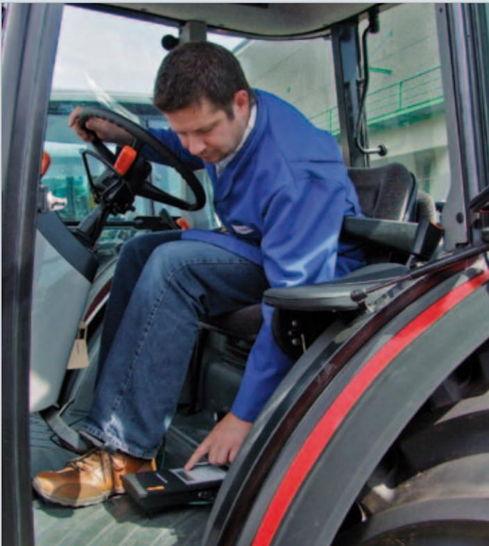
The VZM 300 measurement unit is simply placed on the floor of the vehicle for the measurement
