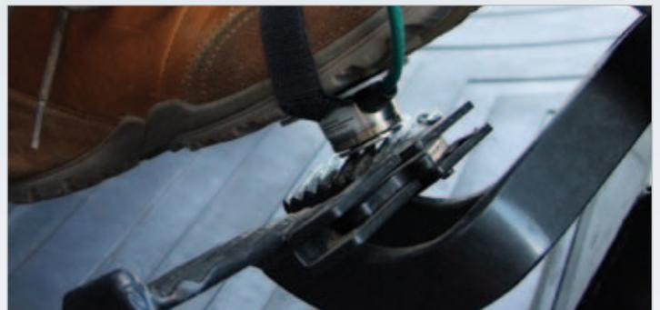
Additional measurement value recording using a pedal force sensor during the brake test
