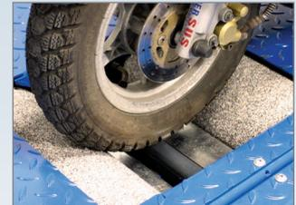
Roller set with lifting bar and automatic roller brake
