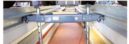
Long support tubes (400, 600, 800 mm) can be pushed through from below and thus enable a very high support range within the pit.
