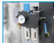
Option: The air filter function in the maintenance unit protects the jack.
