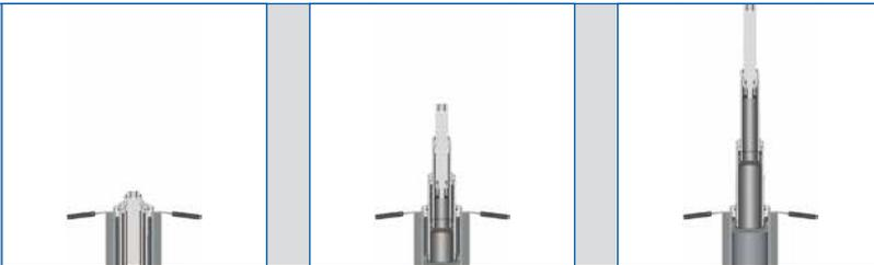
Telescopes travel continuously and at the same high speed along the entire lifting and lowering path. Rapid control to the load point and back is used with synchronised cylinders in all telescopic stages. These features thus ensure completely safe, solid and jerk-free use.
