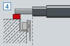
Variant with wooden block additional elevation
