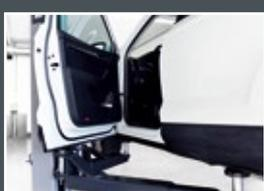
Large door opening for easy exit from the vehicle thanks to 45° rotated columns (MA STAR 3.5 A).
