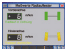
Side slip test Clear display of the directional stability of the vehicle axes.
