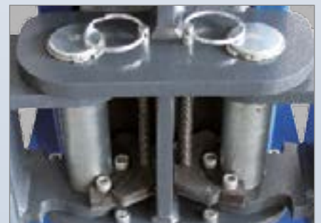
Automatic support-arm restraint with fine adjustment and manual release
