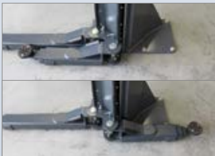
180° pivoting range of the short support arms provides maximum take-up area. This allows the support arms to be moved to the take-up points via the shortest possible route.
