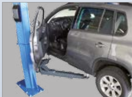
Support arms with asymmetric design, providing optimum door clearance
