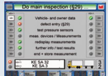
Predefined test sequences reduce the effort required to operate the equipment to a minimum.
